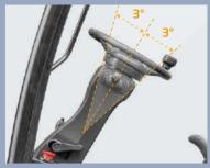
The angle of the hand wheel is adjustable
